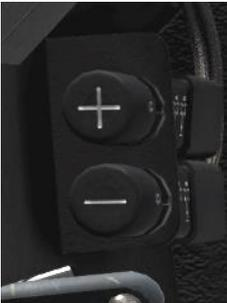
The DEST BUT can be incremented or decremented using the DEST BUT Increment/Decrement buttons on the left of the front dash
