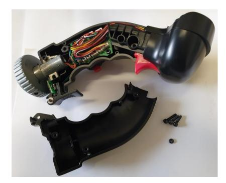
3) Disconnect all the 12 connectors and unscrew the 2 Allen screws shown on the picture:
