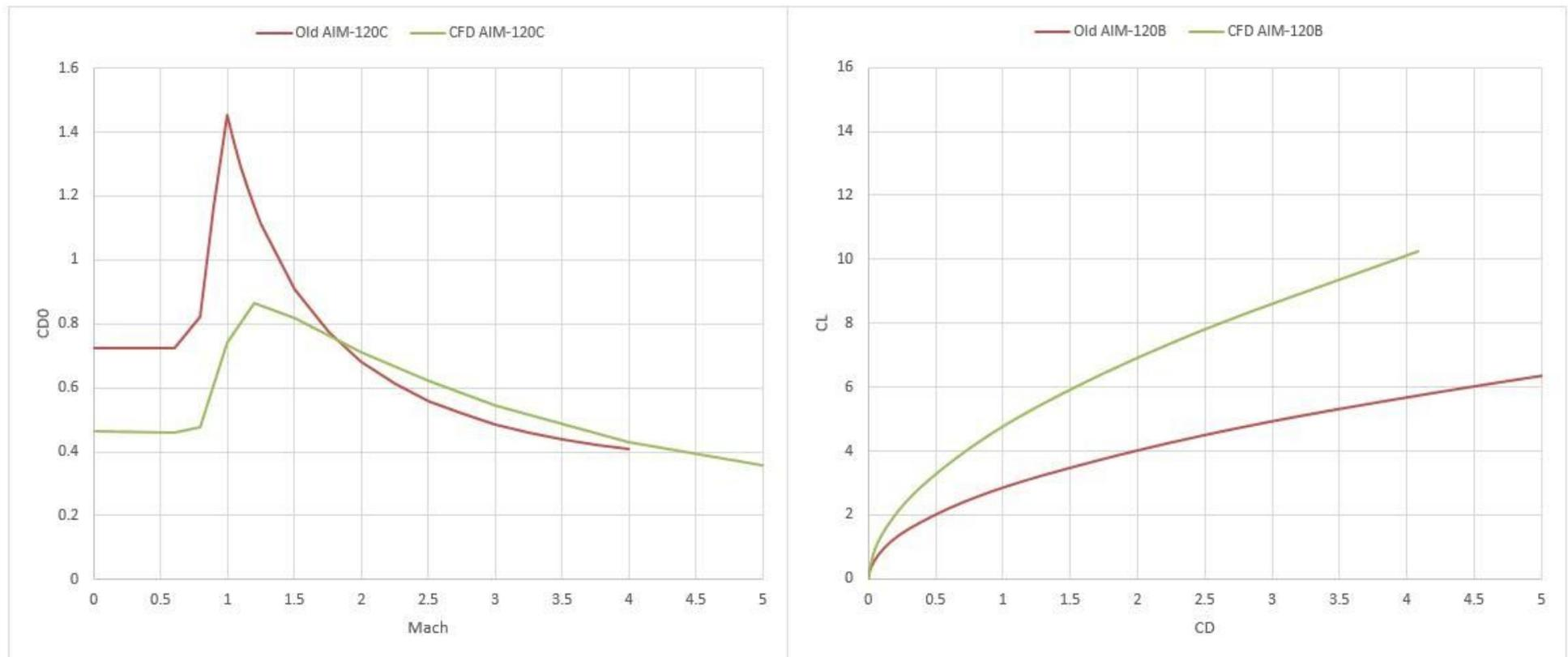
Figure 1. Missile zero-lift drag and induced drag polar at Mach 2.
