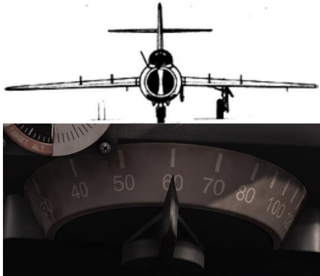
WINGSPAN OF A MIG-15BIS 10 m = 32 ft (VALUE TO ENTER IN GUNSIGHT WINGSPAN)
